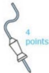
Heated core probe w 4 measuring points
