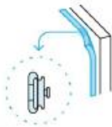
Magnetic door gasket removable w/o tools
