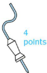
Heated core probe w 4 measuring points
