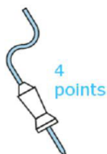
Heated core probe w 4 measuring points
